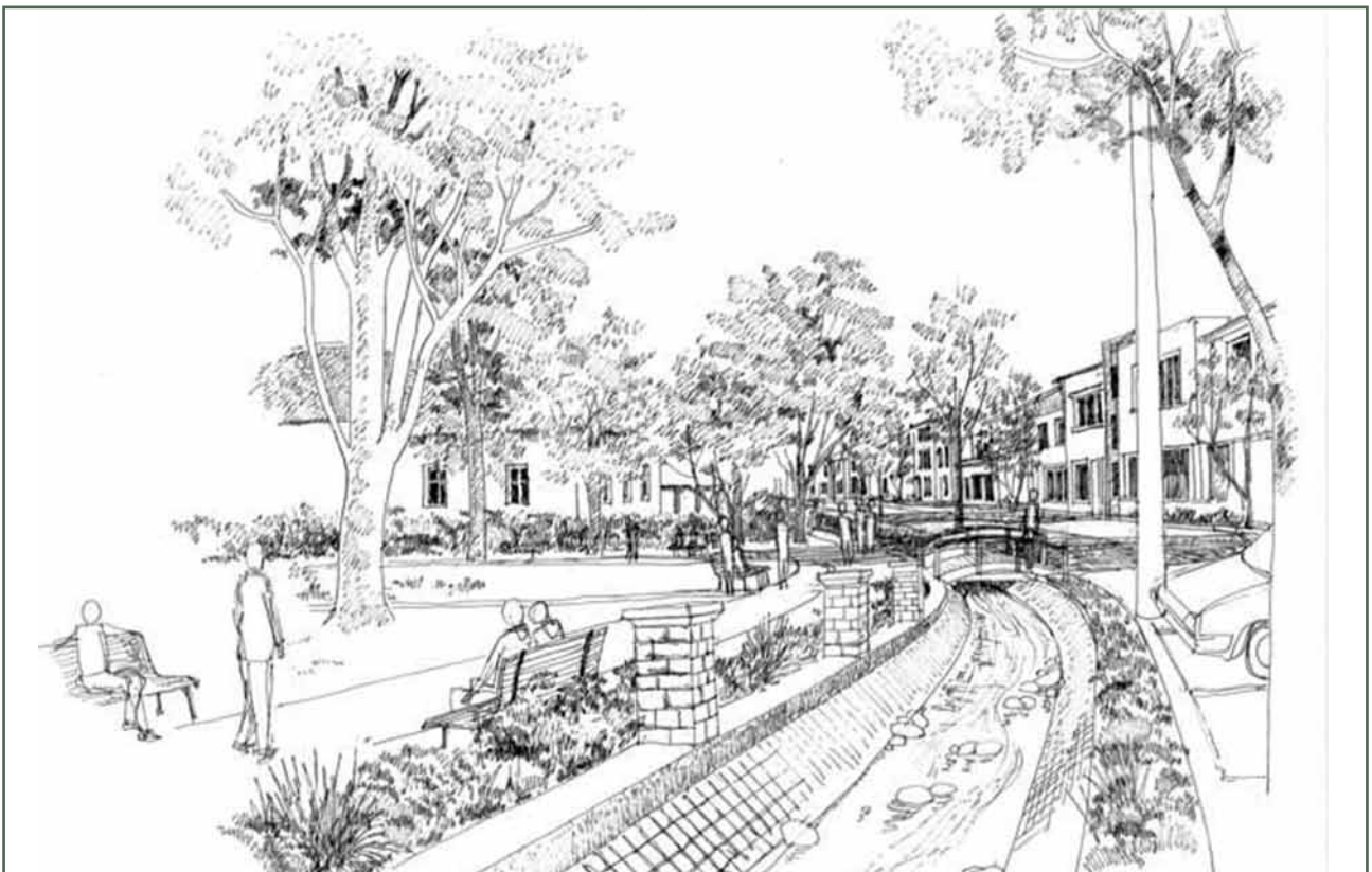
Proposal for existing irrigation channel that seeks to add riffles and river washed rocks in the channel to add movement and sound to the qualities offered by the channel to its surroundings and frame it with appropriate riparian vegetation.
